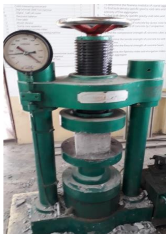
Fig.3: Concrete cube test in Compressive test machine(CTM)
