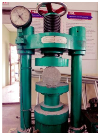
Fig.5: Concrete cylinder in CTM
