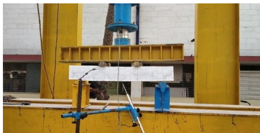
Figure 11: BMW with Meta Kaolin under Four Point Load
