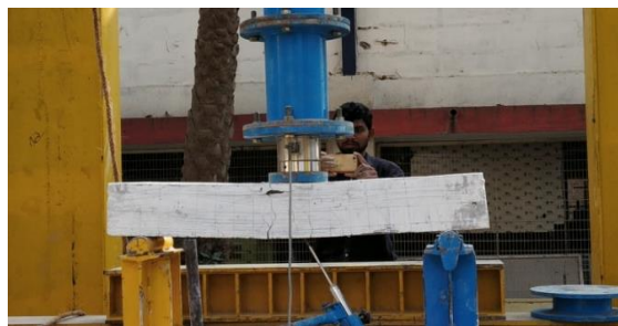
Figure 10: Control Specimen under Three Point Load
