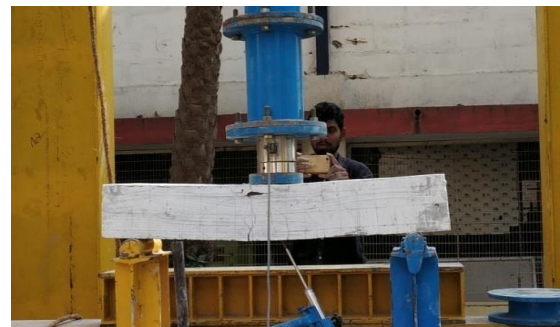
Figure 9: BMW with Meta Kaolin under Three Point Load
