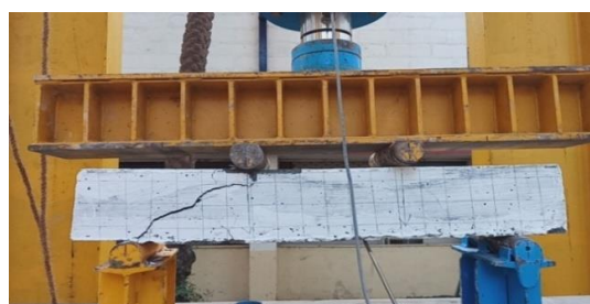
Figure 12: Control Specimens under Four Point Load
