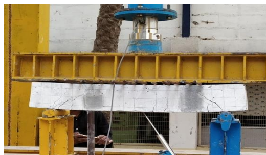
Figure 13: BMW with Meta Kaolin under Uniformly Distributed Load
