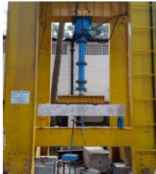
Fig. 10: Experimental set up under 4-point loading
