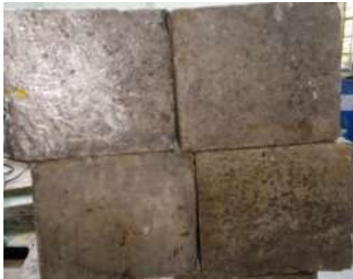
Fig. 8 : Sulphate attack (MgSO 4 )
