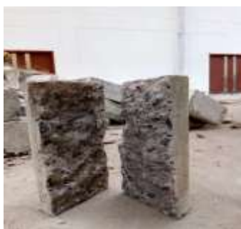
Fig. 10: Splitting of cylinder after testing
