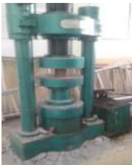
Fig.13: Motor cube testing CTM
