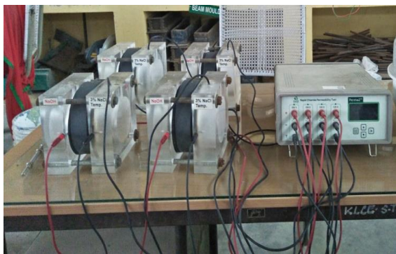
Figure 3: Rapid chloride penetration test equipment
