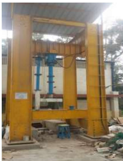
Fig:4: Beam Column Joint setup
