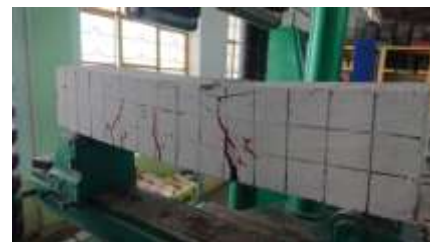
Fig. 13 Failure of Beam
