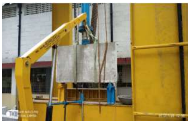
Fig. 3: Loading Frame with Deep Beam
