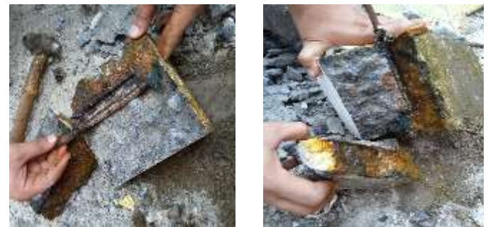
Fig. 4: Formation of corrosion and cracks
