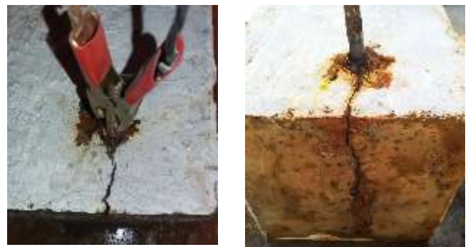
Fig. 4: Formation of corrosion and cracks
