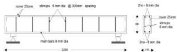
Fig. 2(a): reinforcement details for pt = 0.25%
