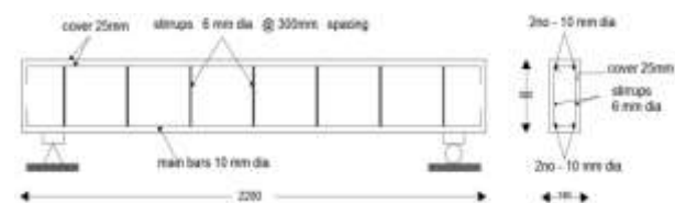
Fig. 2(d): reinforcement details for pt = 0.39%
