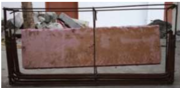
Figure 5: Reinforcement details of 0.15% - 300 mm deep beam
