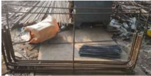
Figure 3: Reinforcement details of 0.15% Control deep beam
