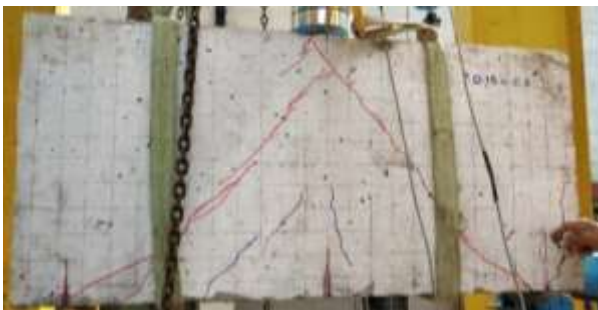
Figure 13: 0.15% CS at Ultimate loading condition
