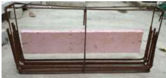
Figure 4: Reinforcement details of 0.15% - 200 mm deep beam
