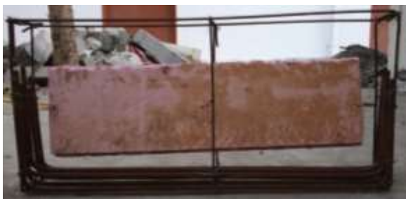
Figure 6: Reinforcement details of 0.15% - 400 mm deep beam
