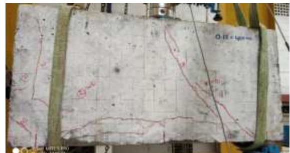
Figure 16: Ultimate loading condition 0.15% 400 mm deep beam
