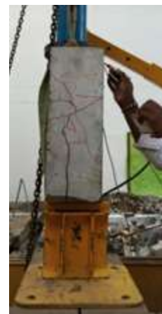
Figure 17: Ultimate loading condition 0.15% 400 mm deep beam side view
