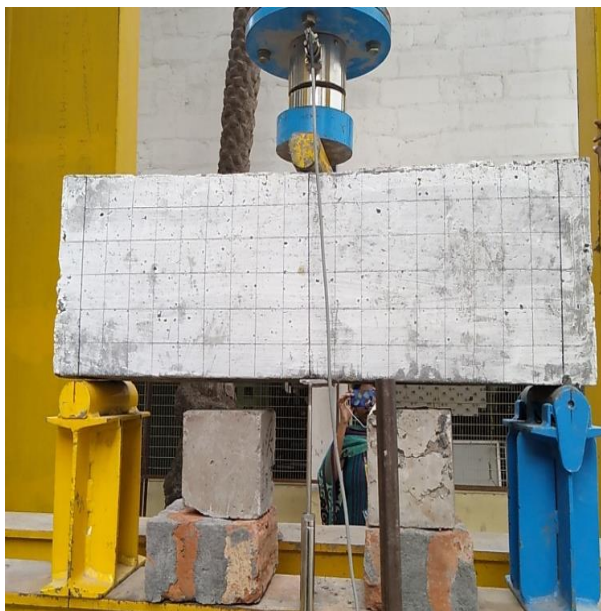
Fig. 5: Three Point Bending Test
