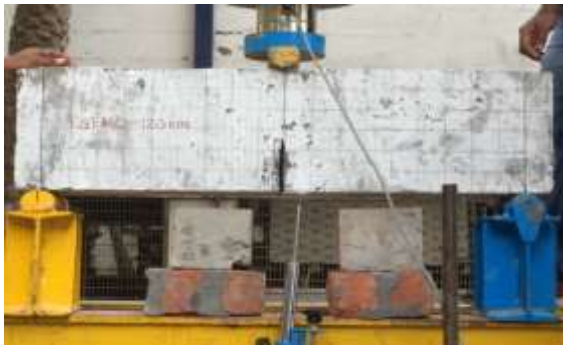
Fig. 4: Test setup of a 120 mm notched SFRC beam under three point loading
