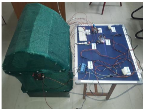
Fig. 11. Working Model of Intelligent Greenhouse Environment Monitoring and Automatic Controlling System Using IOT
