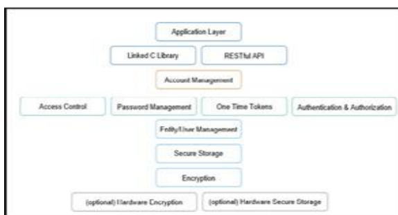
Figure 3. Libsecurity– Security Modules
