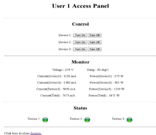
Fig.10 Controlling and Monitoring of all three devices
