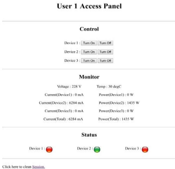
Fig.8 Controlling and Monitoring of Air Conditioner
