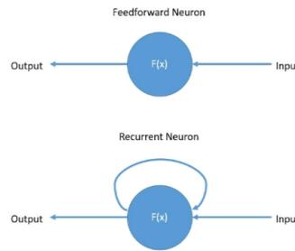
**Fig 4 . Basic structure of a Recurrent Neuron**
