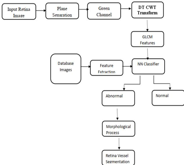
**Fig 5. Process flow diagram of Image processor with Pre-processing, feature extraction and Classifier.**
