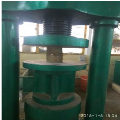
Fig 2: compressive testing on CTM.
