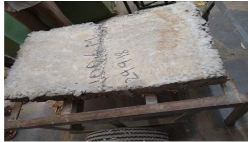
Fig.7. crack pattern of specimen
