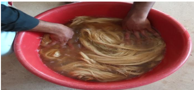
Fig.1 Chemical treatment on Sisal Fiber
