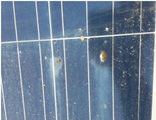
Figure 1a: Shading due to Bird's Feces
