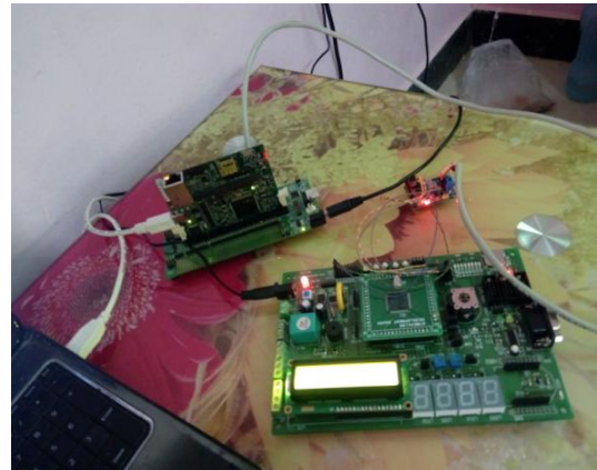
Fig. 4 CAN Transceiver (Sender – At mega 128 Microcontroller, Receiver – Texas Instrument, CAN Module – MCP2515)
