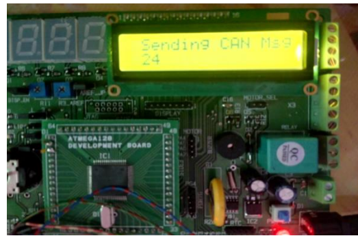
Fig. 3 Sending Data (Room Temperature) from ATMEGA 128 Microcontroller
