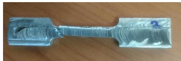
Figure 7: Sample 1 after Tensile Test
