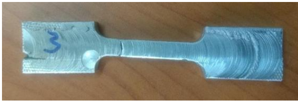
Figure 8: Sample 2 after Tensile Test
