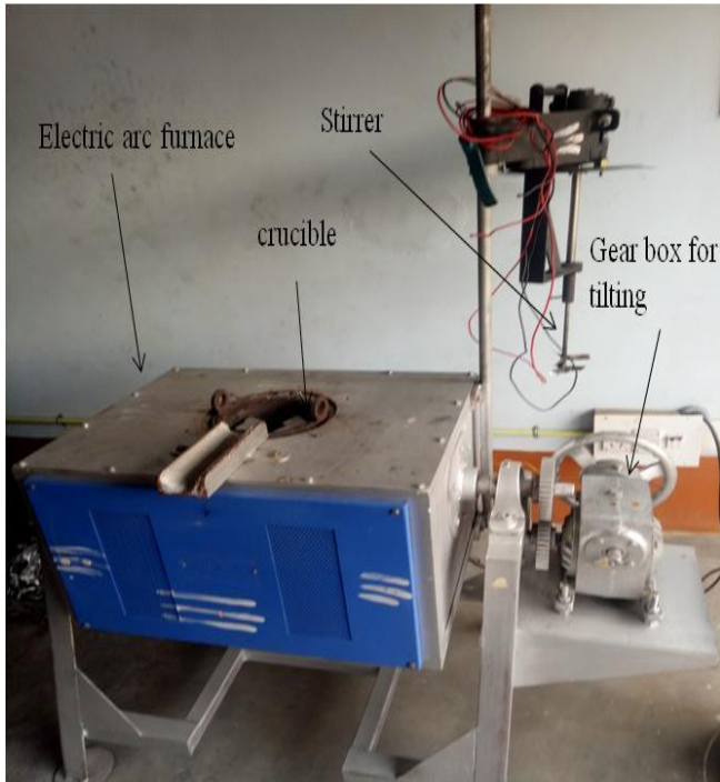
Fig. 1: Stir casting setup
