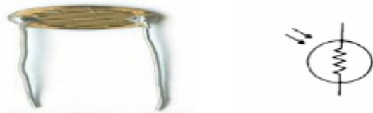
Fig 2: LDR and Circuit Symbol of LDR
