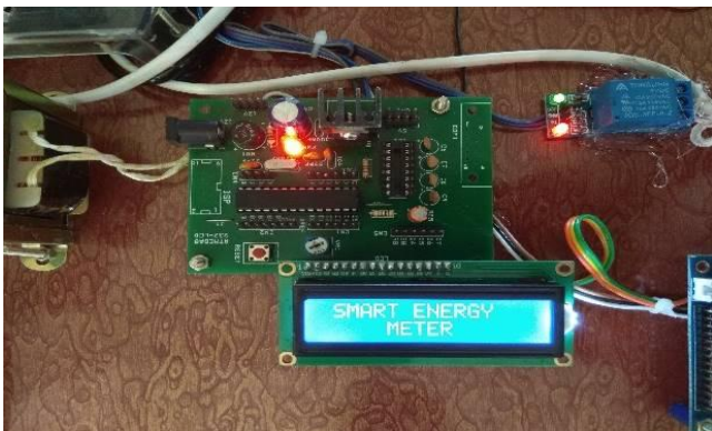
of Smart Meter is shown in Fig.2 Fig.2. Smart meter Hardware setup when it is switched ON. After the indicating the Turn ON condition of the smart energy meter the Smart energy meter checks the signal strength of the GSM module connected to the Smart meter which is shown in Fig.3. Once the Signal strength is good the Smart meter is ready to send and receive messages which is shown in Fig.4.
