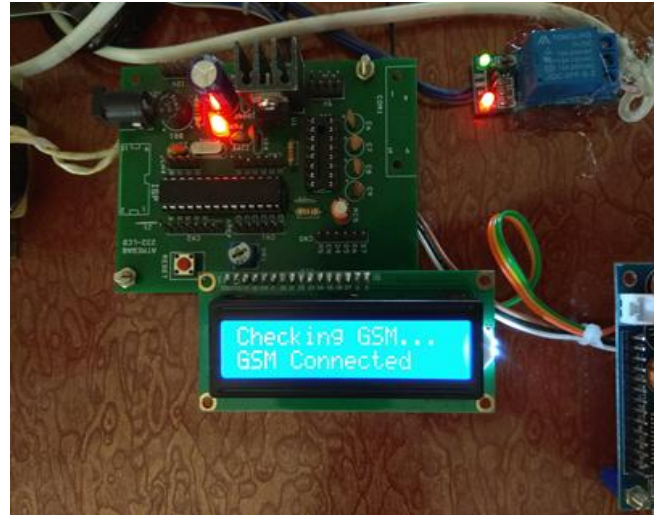
Fig. 4. Establishment of network connection. Once the network is established the smart energy meter is ready to send and receive messages and a test message is initiated through SMS in order to check the proper functioning of the Smart meter which is shown in Fig.5. The test message received by the users is shown in Fig.6
