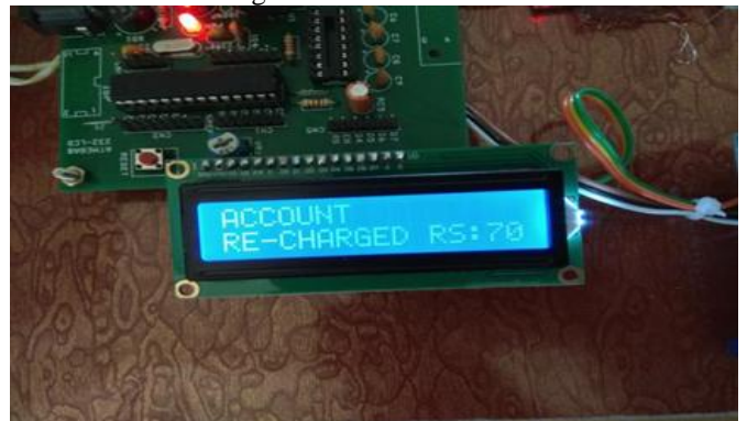
Fig.11. Acknowledgement for the recharged amount. The presence of Anti-Theft system in the smart energy meter protects the users by indicating them if unknown loads are connected to their system. This helps in encrypting of the data present in the device and provides privacy for the customers. Once the Theft is detected the smart energy meter send SMS to the user about the theft through the GSM module present in the hardware setup which is shown in Fig.12.
