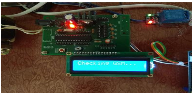
Fig.3. Checking of Network strength.
