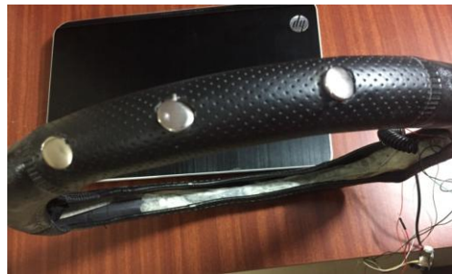
Fig.5 The steering wheel along with the GSR sensor
