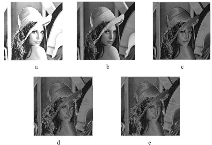
Fig. 9: Foreground detection using proposed accurate-approximate subtractors. (a). Input image1 (b). Input image2 (c). output image after exact subtraction (d). Output image using ApXs1 (e). Output image using ApXs3 .
