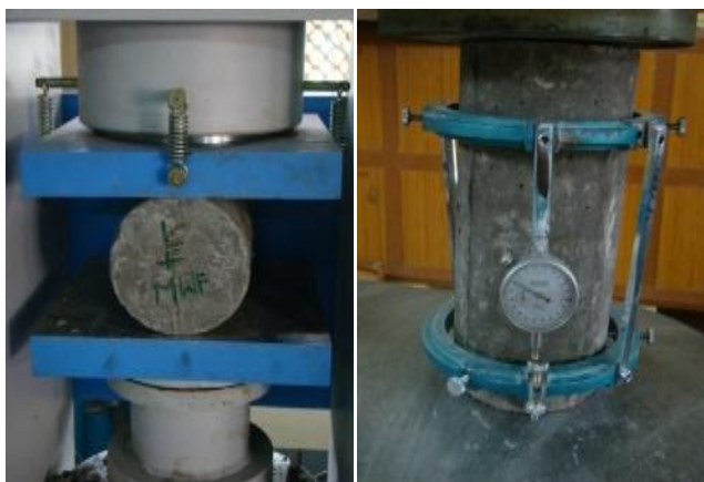
Fig. 3 (a) Split tensile strength test (b) Modulus of Elasticity test
