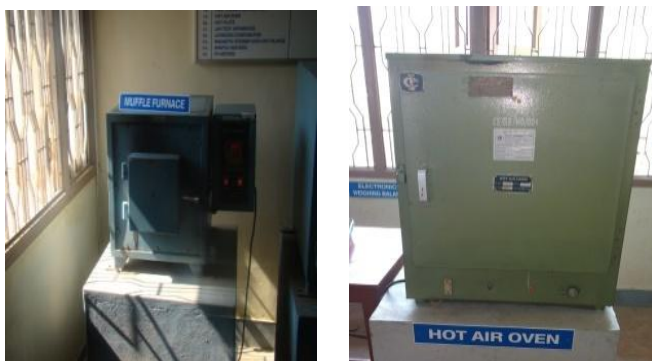
Fig. 4. (a) Muffle furnace –Elevated temperature test (b) Hot air oven-water absorption test
