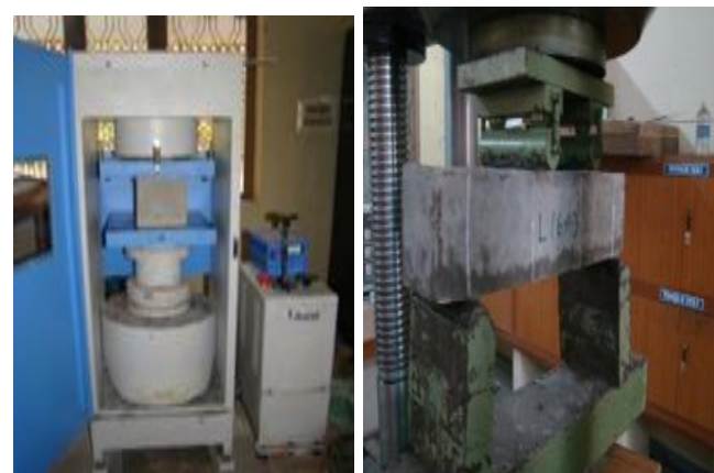
Fig. 2. (a) Compression test (b) Flexural testing setup
