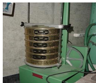
Fig: 3.3 Sieve analysis setup
