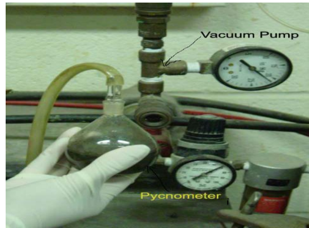
Fig 3.5 Specific gravity test setup
