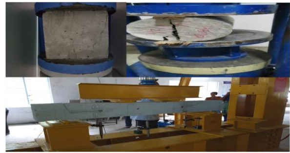
Figure No: 4 Testing of geopolymer concrete specimens
