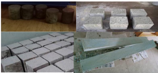
Figure No:3 Geopolymer concrete specimens Curing at different environments
