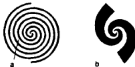
Fig. 2. Two arm equiangular spiral antenna
