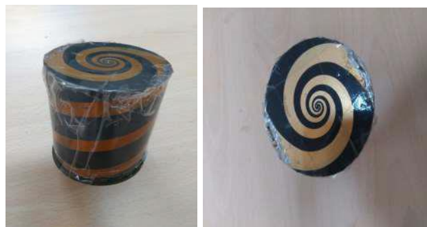
Fig. 12. Practical helix spiral and spiral antenna
