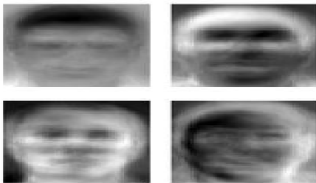
Fig 2: Eigen face calculated from ORL database
