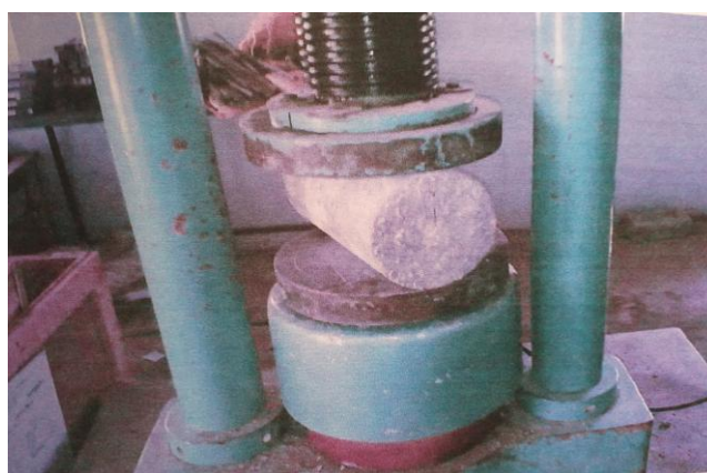
Fig. 7. Split tensile test
