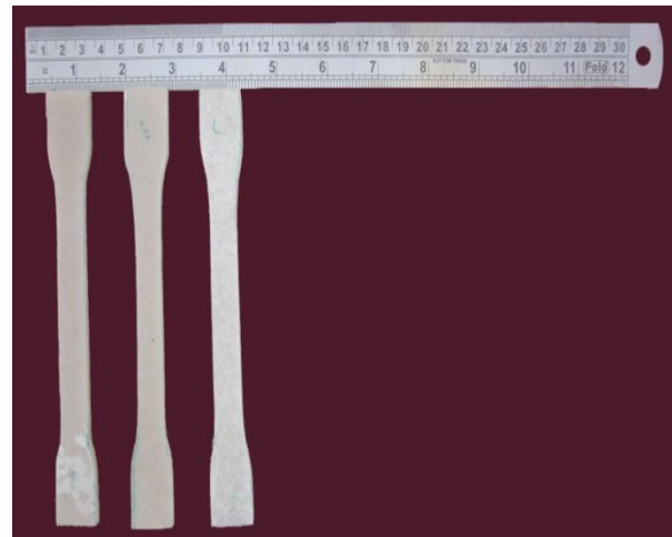
Fig. 1: Specimens for tensile test
