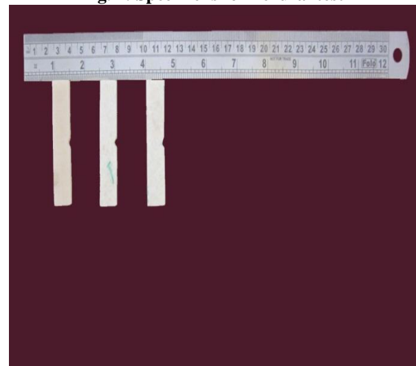
Fig. 3: Specimens for impact test
