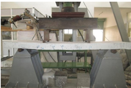
Figure 8. Simply supported block specimens post Failure
