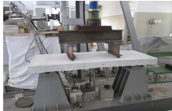
Figure 3. Loading Set up for Simply Supported Slab
