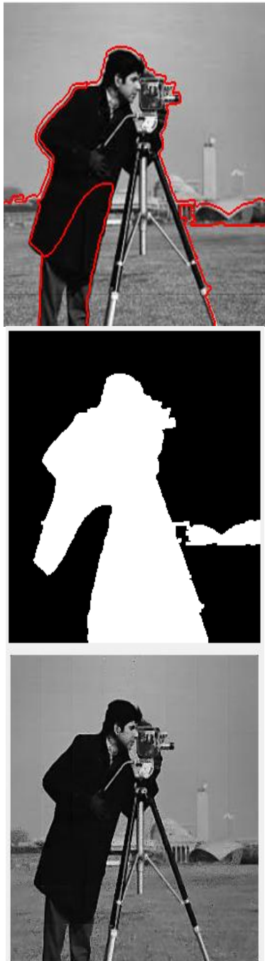
Figure 3(a): Random walker segmentation Figure 3(b): Texture boundary segmentation Figure 3(c): Denoised image using Mask-NHA
