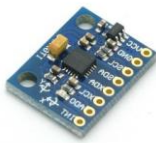
Fig. 2: InvenSense MPU-6050 gyro sensor which is used for measuring tilt angle of the vehicle
