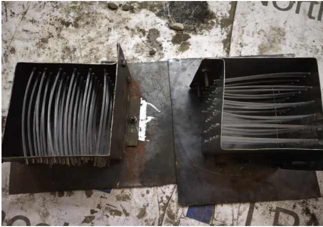
Fig 1: Molds made of steel, drilled on two opposite faces.
