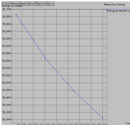
Fig. 2: Residual energy in proposed method for 50, 100,150 and 200 nodes
