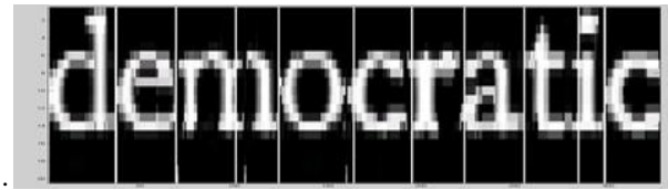
Fig. 10: Predicted: dennocratic. The character 'm' was predicted as a sequence of two 'n' characters.
