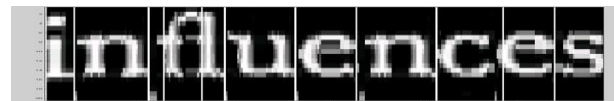
Fig. 11: Predicted: ininfluoes. The system interpreted the character 'c' and the beginning of character 'e' as an 'o', and it predicted an extra 'i'.
