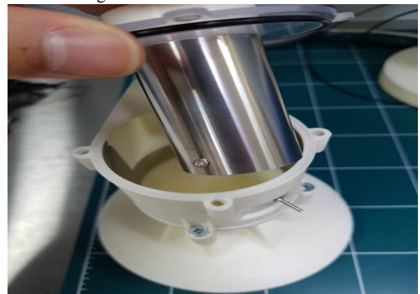
Figure 3. Cylindrical SUS electrode connections
