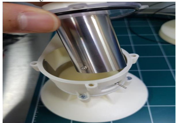
Figure 3. Cylindrical SUS electrode connections
