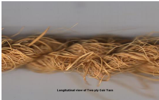
Figure.4. Longitudinal Image Of Two Ply Coir Yarn.
