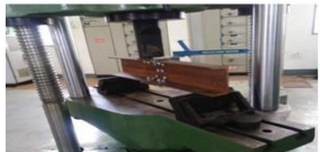
Figure 5. Experimental set up for specimens with and without splice connections
