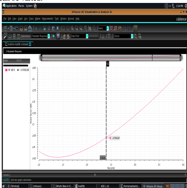
Figure 4. Noise figure of 45 nm LNA with CS with inductive load
