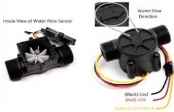
Figure.3 Flow Meter Internal Structure
