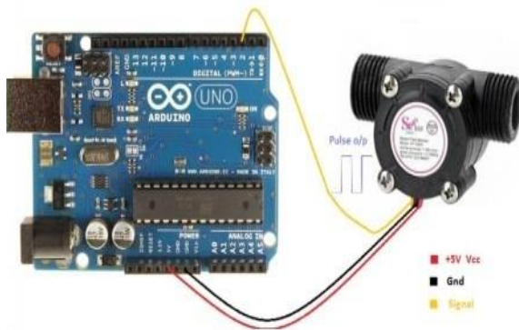
Figure.4 Flow Meter and Arduino Interface
