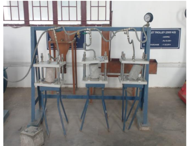
Fig. 3. Water Permeability Test
