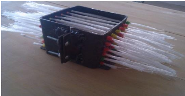
Fig.2.Casting of Transparent Concrete
