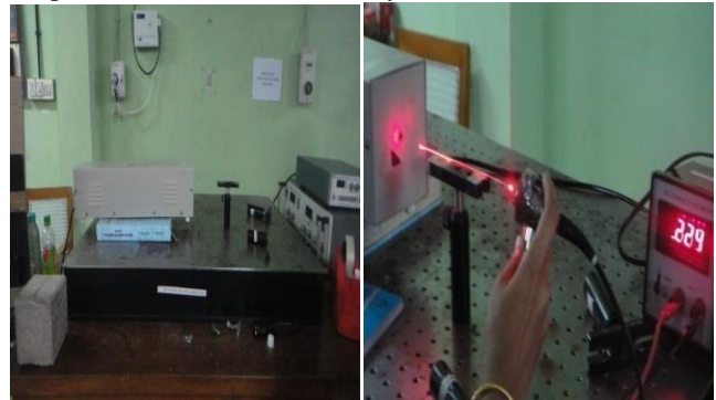
Fig.4. Experimental set up for the Determination of Attenuation of Fiber
