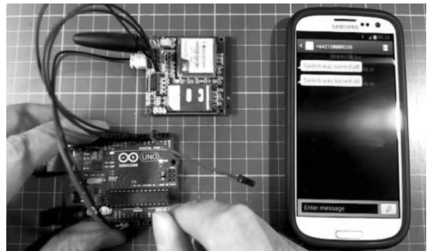
Fig (3) GSM Transmitting the Information
