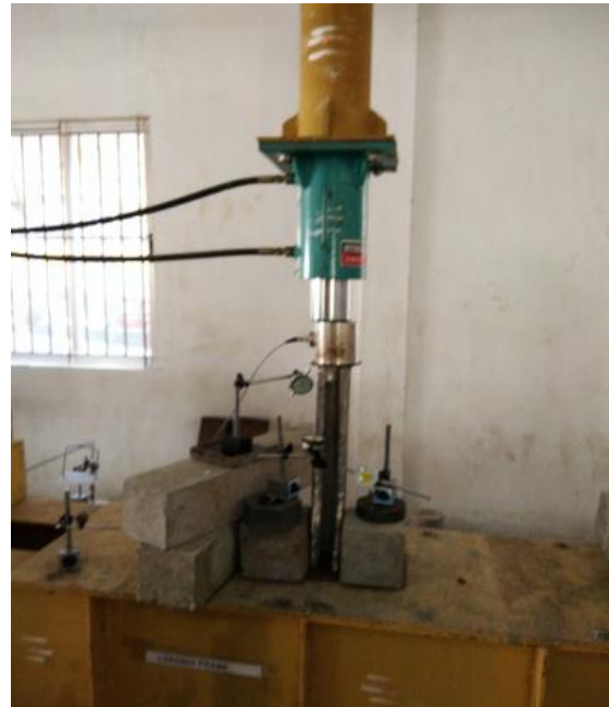
Fig.4testing of a CFS column
