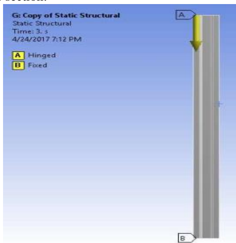
Fig.3 Boundary and Loading Condition
