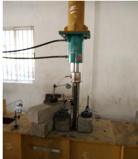
Fig.4 testing of a CFS column
